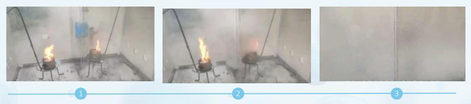
When the ambient temperature reaches the thermal decomposition temperature of the temperature-sensitive material inside the product, the material decomposes to produce a large amount of nitrogen ( $N_2$ ), carbon dioxide ( $CO_2$ ), and nano-scale fire extinguishing particles and other fire extinguishing substances.
